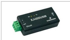
XJ485USB is an optically isolated converter with 2.5kV maximum voltage isolation on data channels. It has a small plastic box with 2 indication LEDs, RX and TX, to quickly monitor the network communication. Power supply directly from USB port.
