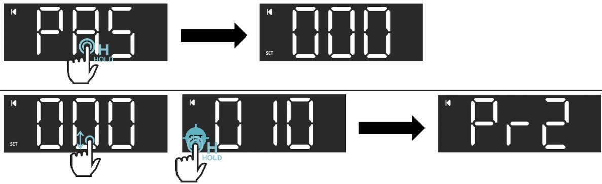
When in the **PAS** menu, it is possible to set the password value by touching the display anywhere (1 or 3 sec depending on par. **bPt**). Use V-swipe on every single digit to modify the value, then confirm the password value pressing the SET icon (1 or 3 sec depending on par. **bPt**).
