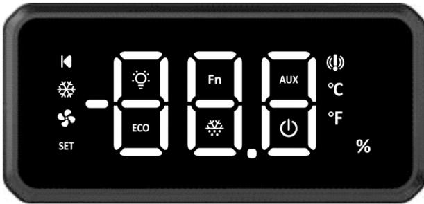
**XH78T** has a capacitive user interface with Full Touch technology. The whole display area is used to interact with the device. Specific gestures are used to enable or disable functions, browse through screens and operational modes and modify the configuration of the device.
