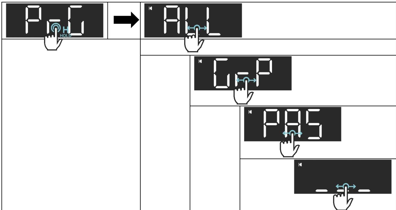
From the PRG screen is possible to unlock the programming menu by touching any area of the display (1 or 3 sec depending on par. **bPt**).
