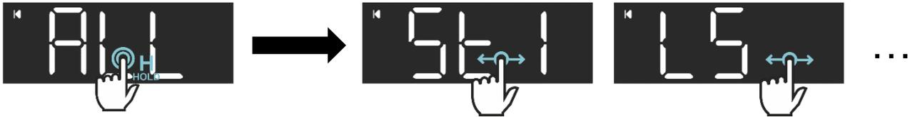
From **Parameter Menu - ALL**, it is possible to enter and browse the list of available parameters by using the H-swipe gesture. All parameters present into level Pr1 are immediately visible. To enter parameters into level Pr2 the password must be inserted.
