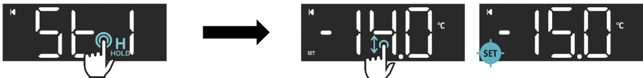
When in **Setpoint Menu St1**, it is possible to enter the **Temperature Setpoint modification** by touching the display anywhere (1 or 3 sec depending on par. **bPt**). Adjust the value through some V-SWIPE gestures on the top of every single digit and then confirm the new value by pressing the **SET** icon. Press the **BACK** icon to exit (come back to the **Setpoint Menu**) without saving.
