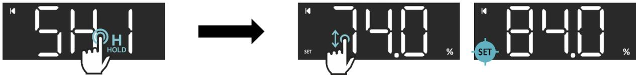
When in **Setpoint Menu SH1**, it is possible to enter the **Humidity Setpoint modification** by touching the display anywhere (1 or 3 sec depending on par. **bPt**). Adjust the value through some V-SWIPE gestures on the top of every single digit and then confirm the new value by pressing the **SET** icon. Press the **BACK** icon to exit (come back to the **Setpoint Menu**) without saving.
