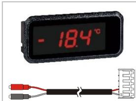
The XH-REP remote display enables the visualization of a second temperature value. A special cable must be used to connect an XH-REP to the controller (code DD200002 00). The remote display usage will disable the serial communication.
