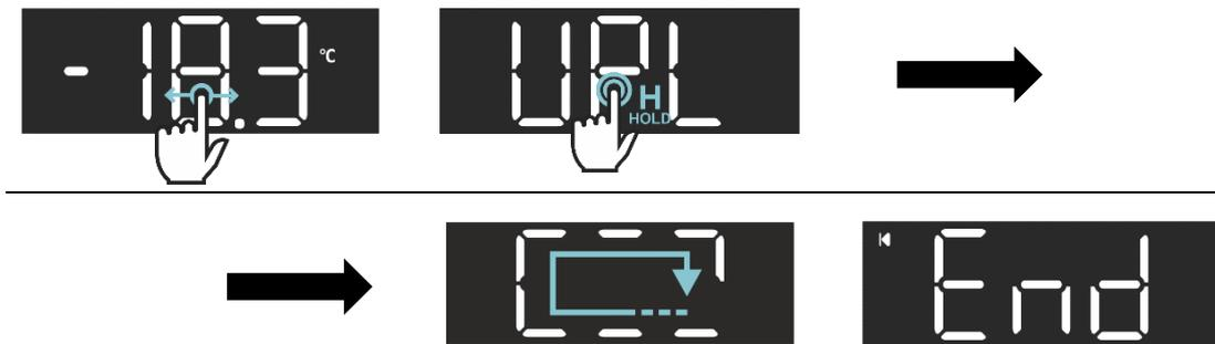
It is possible to use the **HotKey Upload Menu** function to save the current device configuration (parameter values) into the external memory. To do this, follow these instructions:
