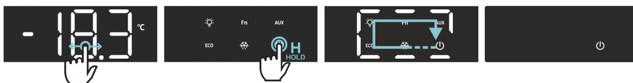
When in **HOME** screen, H-swipe to go to the Virtual Keyboard screen and then touch the **OFF** icon for 3 sec. The beginning of this action will trigger an animation effect (a “snake” moving effect of the frame around the icons). to All outputs and alarms are deactivated in Stand-by mode.
