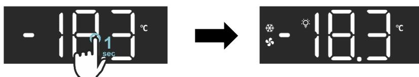
Depending on par. **SC7** it is possible to visualize both the active outputs and functions when in HOME screen. In particular:
