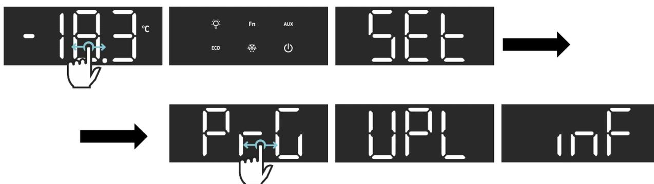
Use H-SWIPE to move through the screens. The logic implements a circular browsing: H-SWIPE to left or right is possible. A programmable timeout is implemented to return **HOME** from any lateral screen.
