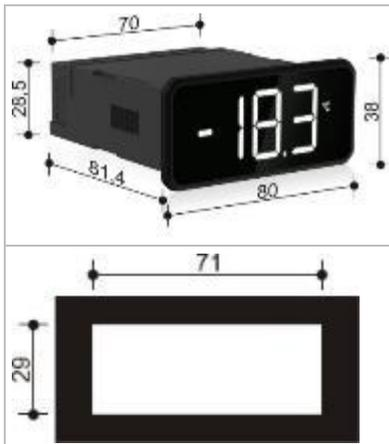
Instrument **XH78T** shall be mounted on vertical panel, in a 29x71 mm hole, and fixed using the special bracket supplied. The temperature range allowed for correct operation is 0 to 60°C. Avoid places subject to strong vibrations, corrosive gases, excessive dirt or humidity. The same recommendations apply to probes. Let air circulate through the cooling holes.
