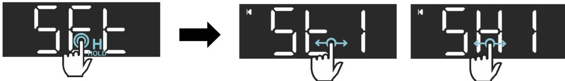
When in **Setpoint menu**, it is possible to enter the **Temperature** or **Humidity Setpoint modification** by touching the display anywhere. The label **St1** or **SH1** indicates that the modification of the temperature or humidity set point is enabled. Use H-swipe to move between temperature (**St1**) and humidity (**SH1**) **Setpoint Sub-Menus**. Press the **BACK** icon to exit (come back to the **Setpoint Screen**).
