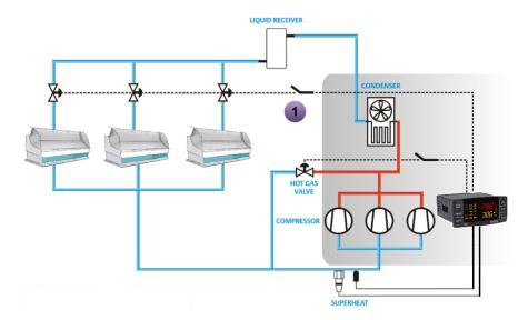
To enable this function set one relay by the parameters oA2 or oA3 or oA4 or oA5 or oA6, as flood protection, El oA4 = Liq, and then connect it to the external device that blocks the cabinet injection.
