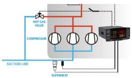
To detect the suction superheat an auxiliary probe among P3 (term. 3-4) or P4 (term. 33-34) has to be set as superheat temperature probe.
