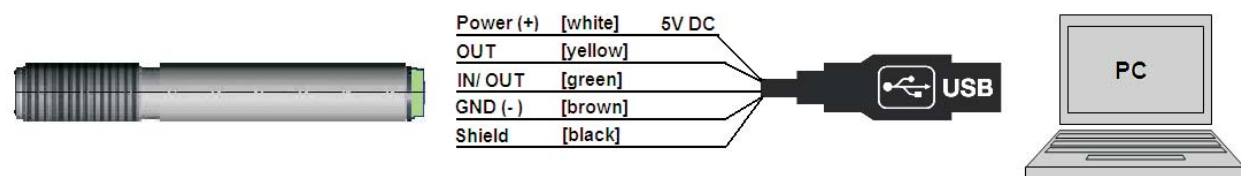
Connection digital with USB adapter cable
