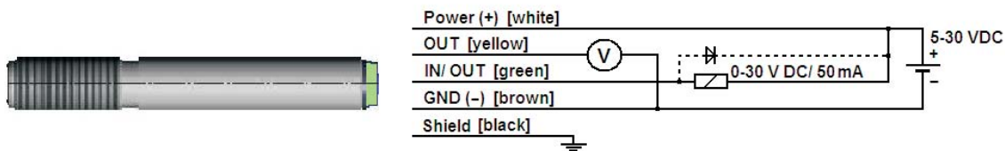
Connection analog with open collector alarm output
