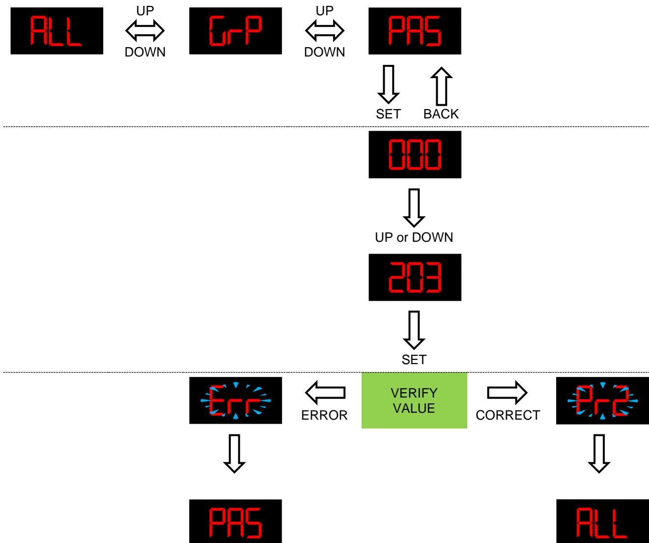
When in Pr2, the label of all parameters in Pr1 will have the “decimal point”.
