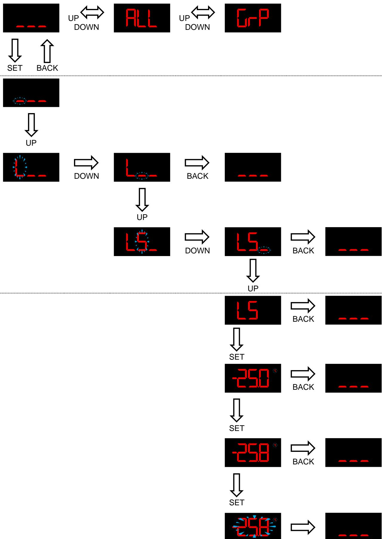
Every parameter is normally identified by a unique label that can have two or three alphanumeric characters. When in the “X9” Screen, it is possible to create the parameter label by selecting every single part of the label itself (first, second and third char). The system is able to drive the user through the available symbols, showing only the available ones to speed up the creation of the label.
