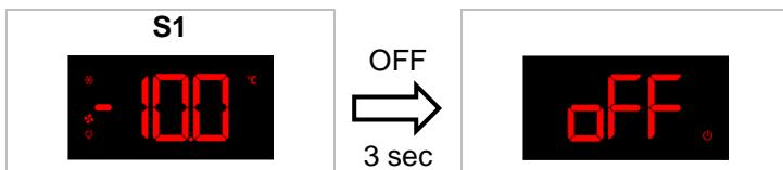
When in **HOME screen**, keep the **OFF** button pressed for 3 sec to activate stand-by mode. All outputs and alarms are deactivated in Stand-by mode. It is possible to visualize the label "oFF" timely through the par. **SC9**. With **SC9=YES**, the label "oFF" will appear 1 sec out of 10.
