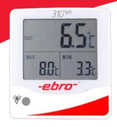
To monitor the sample temperature in the laboratory, but also in microbiological research facilities, a thermometer with minimum and maximum value display is required. In addition, all refrigerators, pharmaceuticals and vaccines, chemicals, greenhouses, blood banks, food and beverage must be monitored and storage facilities monitored. Minimum and maximum values must be recorded daily and documented manually.
