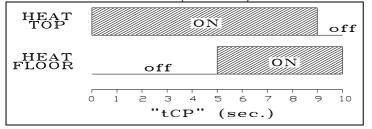
Should the power limiter be activated, by pressing the PW. LIM key, the relative led will light and the controller will ensure that the outputs are never simultaneously on (therefore if the two resistances are equal, the maximum power absorbed is 50%).
