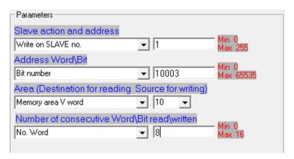
Following example describes the setting for an "EXP" instruction to read from the plc with address "1" of 10 consecutive bit from "data register" DT0 to DT9, keeping read value on area VW0..9.
