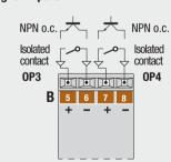
Mhen terminals 5, 6 and 7, 8 are not configured as 0P3 and 0P4 outputs, they can be used as voltage or isolated contact inputs.
