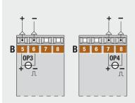
Mhen terminals 5, 6 and 7, 8 are not configured as OP3 and OP4 outputs, they can be used as voltage or isolated contact inputs.
