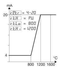
With r t l c greater than r t l h it is possible to obtain a reverse scale.
