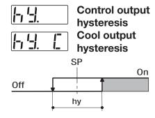
Control or alarm output hysteresis span, set in % of the full scale.
