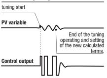
This type is selected when the PV is close to the SP Setpoint. This method has the advantage of a better accuracy in the term calculation with a reasonable speed calculation. The Fuzzy Tuning determines automatically the best method to use to calculate the P.I.D. term, according the process conditions.
