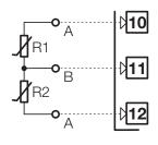
Use wires of the same length and 1.5 mm<sup>2</sup> size. Maximum line resistance: 200/line
