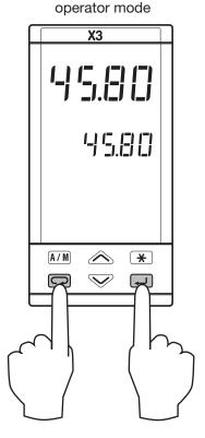
Press simultaneously for 2 seconds
