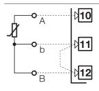
For 3 wires only. Maximum line resistance: 20Ω/line
