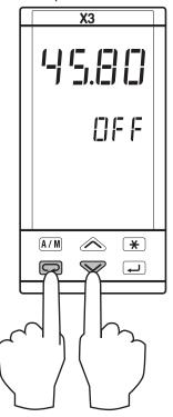
Press simultaneously for 2 seconds
