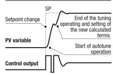
This type is selected when, at the start of the autotune operation, the PV is far from the Setpoint of more than 5% of the span. This method has the big advantage of fast calculation, with a reasonable accuracy in the term calculation.
