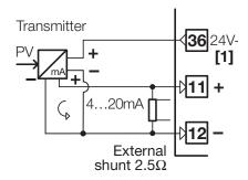
[1] Auxiliary power supply for external transmitter 24Vdc ±20% /30mA max. with no short circuit protection
