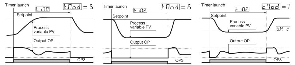
[1] When the Timer is not running the control output is forced to zero, also before the Timer launch
