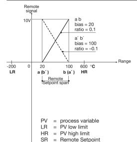
a (a) = SR starting point b (b) = SR ending point If SR starting point is **lower** then the ending point, both expressed in engineering units:
