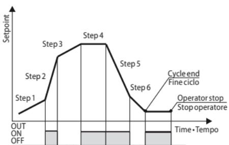
ON/OFF status of the auxiliary output is selectable for each step of each cycle. The status can be selected also at cycle end.
