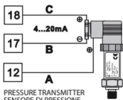
For linear signals 0/4....20mA with **three-wires sensors**
