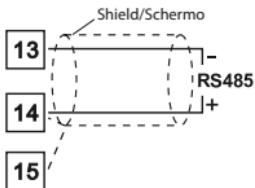
Communication RS485 Modbus RTU.
