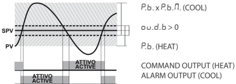
Parameter  $c_o.c.t.$  has the same meaning of cycle time for heating action  $t.c.$ . Parameter  $c_o.o.F.$  (Cooling Fluid) pre-selects the proportional band multiplier and the cooling P.I.D. cycle time  $P.b.\Pi.$ , according to cooling fluid type.
