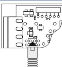
Analogue output in **Volt** configurable as command (Par. *c.outL*) or retransmission of process-setpoint (Par. *rEtr*).
