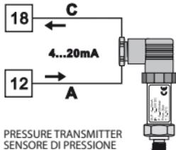
For linear signals 0/4..20mA with **two-wires sensors**
